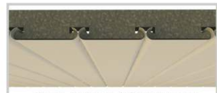
DETAIL SECTION POSITION PANEL
