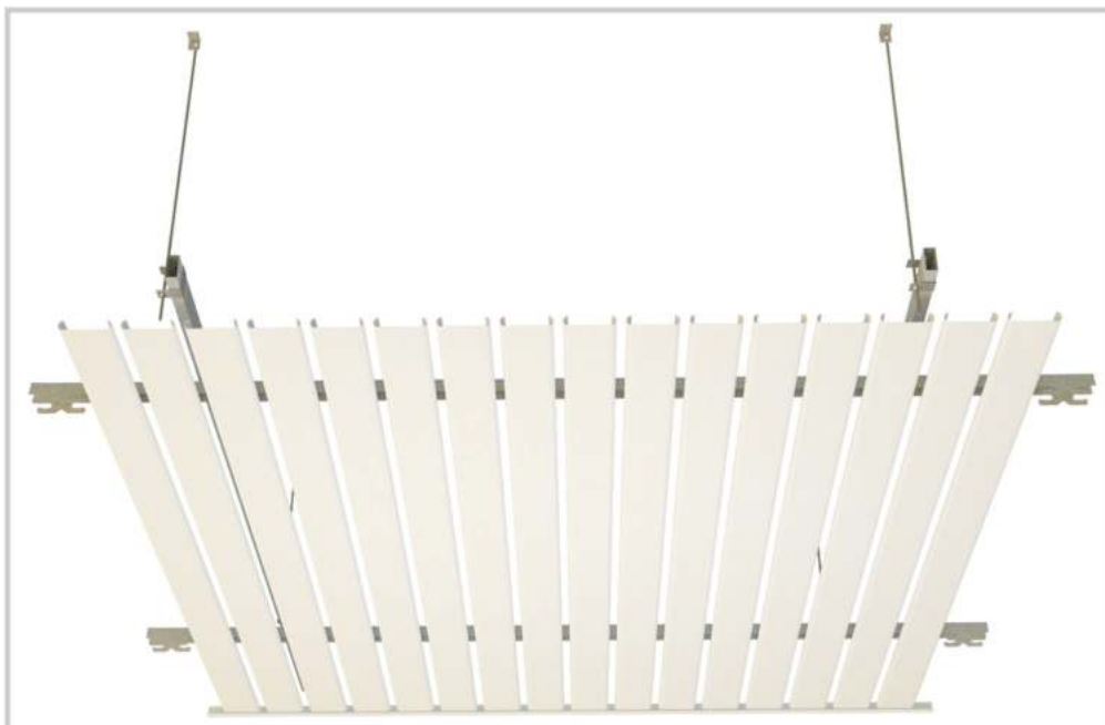
INSTALLATION DETAIL SYSTEM
