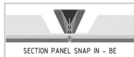
7. SNAP IN, Size 3000mm, Bahan Galvanish Soft #0.70mm
